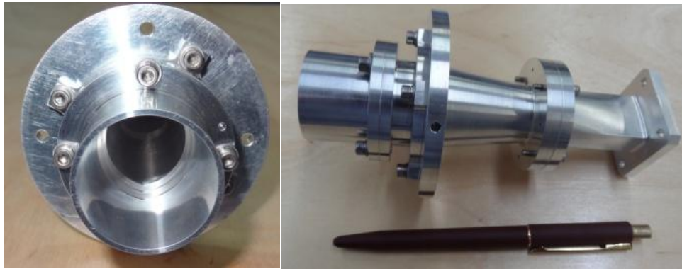
Fig.4.23 Fabricated broadband conjugate matched feed horn
